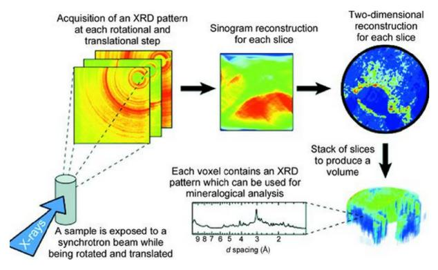
X- ray diffraction tomography can be useful to depict changes during hydration and ageing cement paste!
